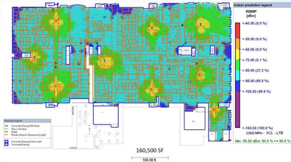
Figure 2. Wall type Sheet rock-Light (incorrect Passing)
