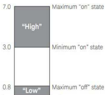
Figure 6. TTL control voltages states (Option 300 and 500)
