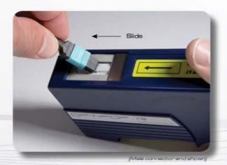
3. With cleaning cloth exposed, slide connector end face in the direction of the arrow.
