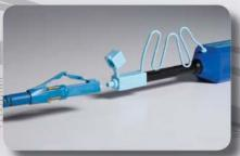
2. Insert connector into the guide cap.
