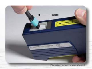
4. Keep connector perpendicular to cleaning surface.
